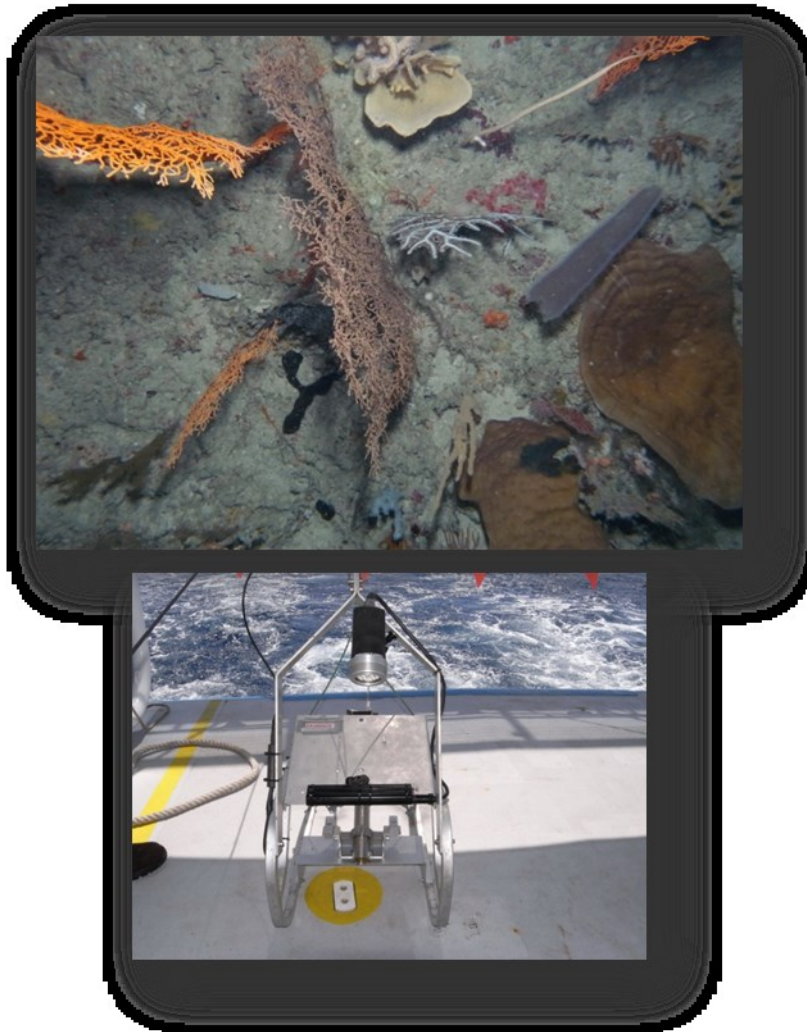
Figure 3. The AIMS towed video system tow body with mounted video camera and down-ward facing camera for stills (lower), with an example of a still photo taken just above the sea floor (above).
